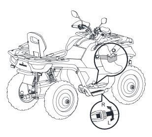
The foot brake lever adjusting nut is located at the bottom of the vehicle near the foot brake lever. The stroke height of the foot brake lever can be adjusted by twisting the foot brake lever nut.
